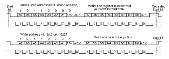
I2C communication protocol with the MD03 module is the same as popular eeprom's such as the 24C04. To read one or more of the MD03 registers, first send a start bit, the module address (0XB0 is the base address) with the read/write bit low, then the register number you wish to read. This is followed by a repeated start and the module address again with the read/write bit high (0XB1). You now read one more registers. The MD03 has 8 registers numbered 0 to 7 as follows;
